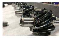
Gears to be protected with wear-resistant coatings.
