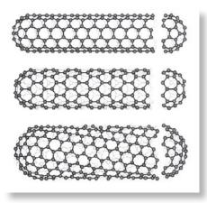
Computer-generated schematic of three types of carbon nanotubes. The diameter of the nanotube in the center of the picture equals approximately 2 nanometers. Illustration courtesy R. Smalley Group, Rice University.
