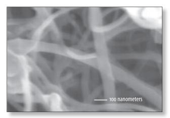
Bundle of multi-wall nanotubes via scanning electron microscopy. The bar at the bottom of the picture represents 100 nanometers. Image courtesy Russell E. Gorga, North Carolina State University.
