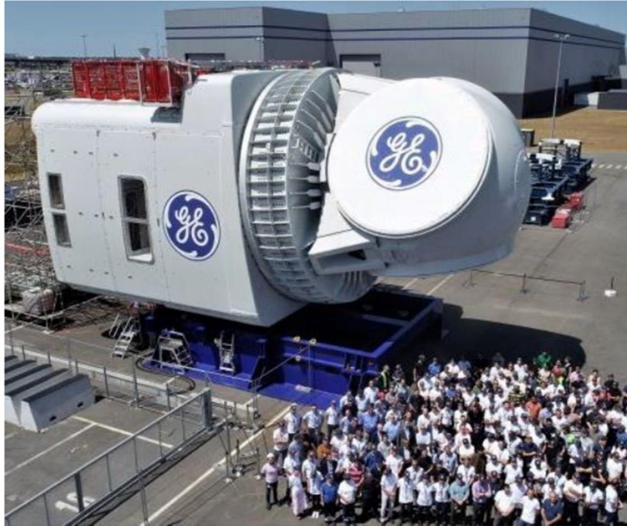
GE Haliade-X nacelle: 14 MW, 220m (721 ft) rotor, ~600 tons.
